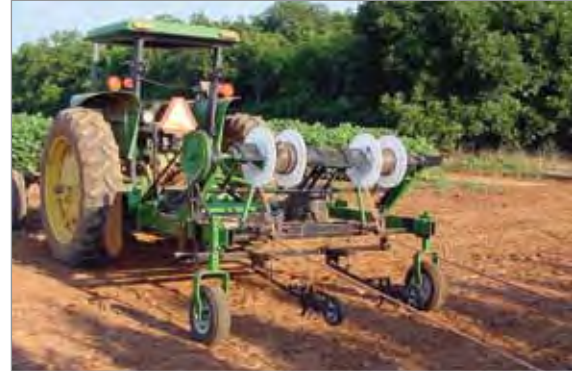
System used to install surface drip tape.
